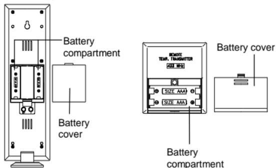
1. First, insert 2 x AA, IEC LR6, 1.5V batteries into the Weather Station. Once the batteries are in place, all segments of the LCD will light up briefly. Then the indoor temperature and humidity, the time as --:-- , and the weather icons sun and clouds will be displayed. If the indoor temperature and humidity are not displayed after a few
