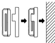
1. Mark the wall using a pen through the holes in the holder to obtain the exact drilling position.
